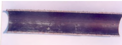
CORROSION OF CONDENSER TUBE WITH HIGH ORGANIC WATER
