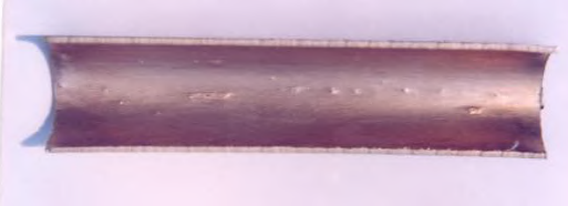
CORROSION OF CONDENSER TUBE WITH HIGH ORGANIC WATER
